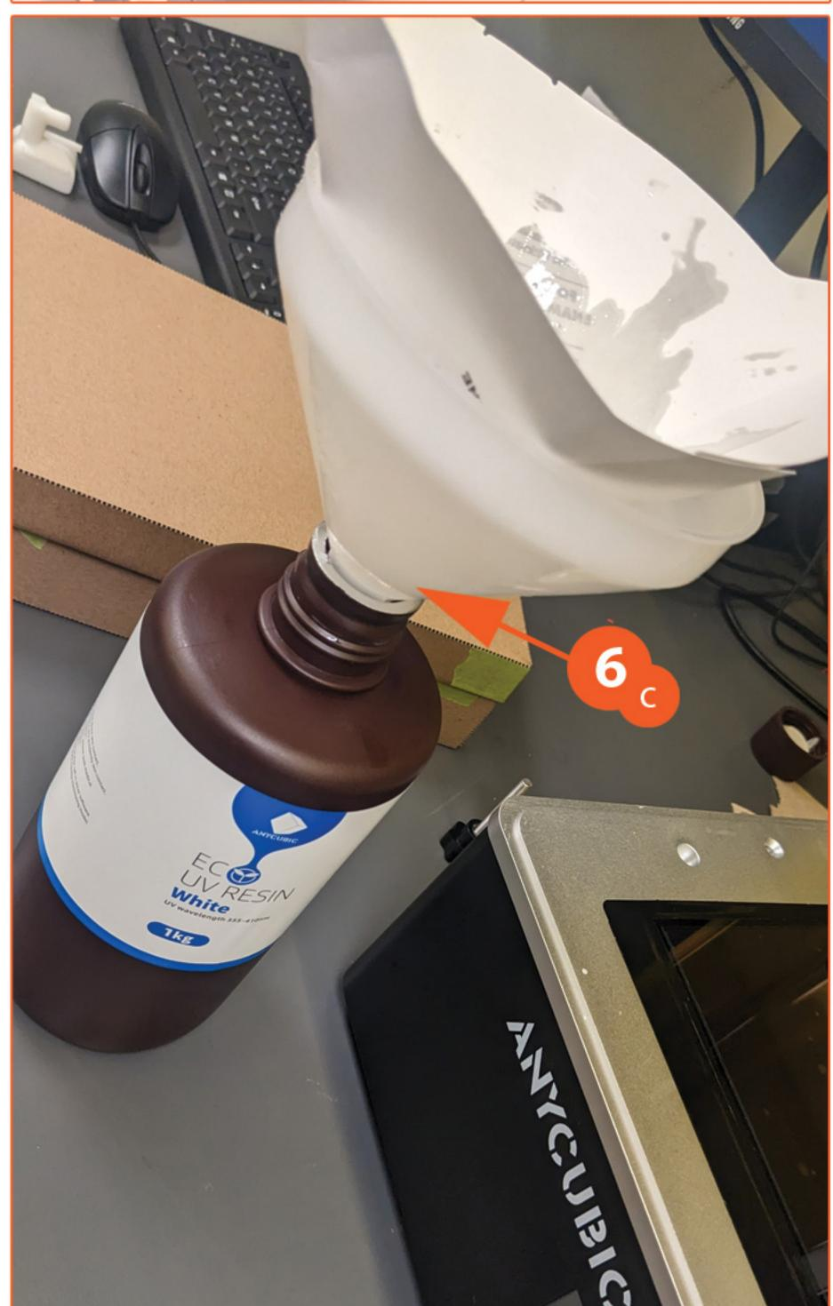
Rotate the printer around to access the Resin bottle.
