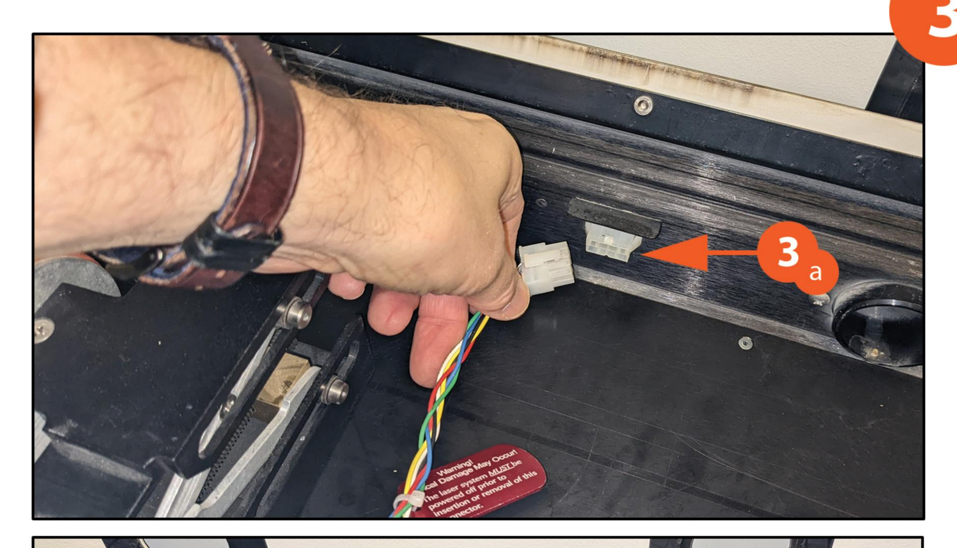
3a - Take the wire harness/plug and insert it (tab side up) into its socket at the middle/bottom/back of the laser bed area.
