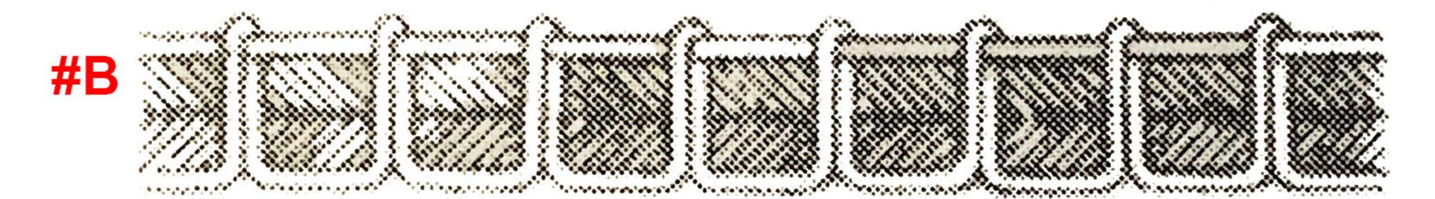
Stitch is bad, loop is at the top of the materials. Turn The thread tensioner counter clockwise (or tighten the tension on the bobbin - #1).
